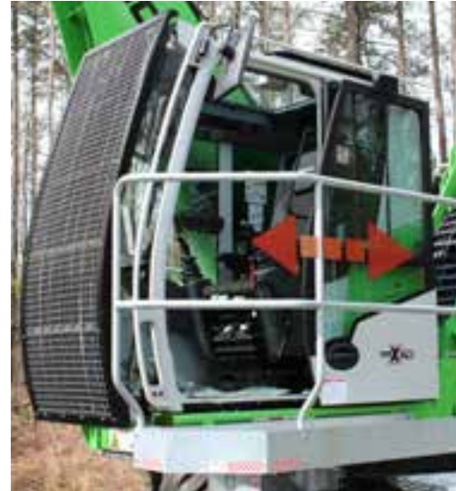
Maxcab's sliding door and guarded permanent catwalk provides the safest entry and exit in the industry.
