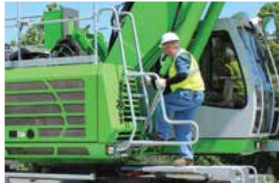
Safe access to the upper deck is achieved with a permanent 3-point contact ladder with railings.
