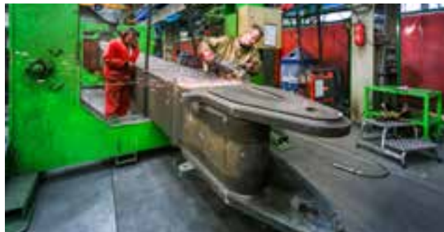
Fabricating booms and sticks in our own shops lets SENNEBOGEN eliminate welding stresses inside the box structure and maximize service life.
