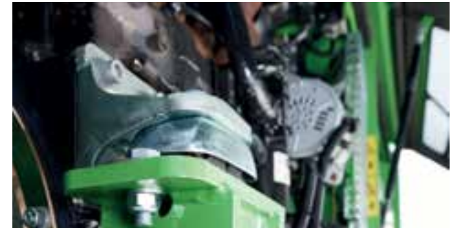
Low-vibration engine mounting reduces wear on components and lowers sound levels.
